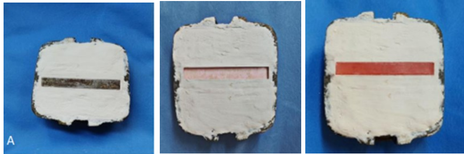
Figure 1: Steps of heat-cured acrylic sample preparation, A. flasking. B. removing of the metal frame. C. deflaxing.
