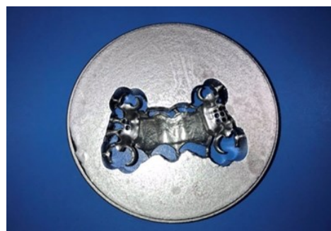
Figure 3: wax pattern after milling
