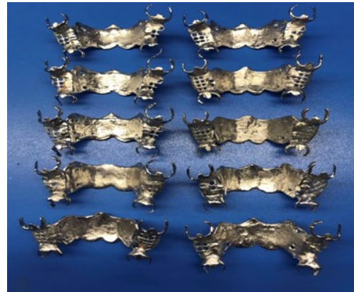
Figure 4: Frameworks after finishing and polishing
