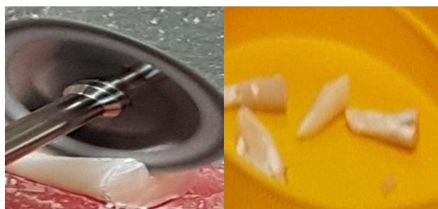
Figure 1: sample preparation by sectioning of root for 2 halves longitudinally from bucco-lingual direction by diamond disc.
