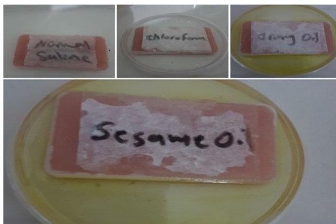
Figure 4: immersing samples in normal saline, chloroform and orange oil and immersing all samples into sesame oil.
