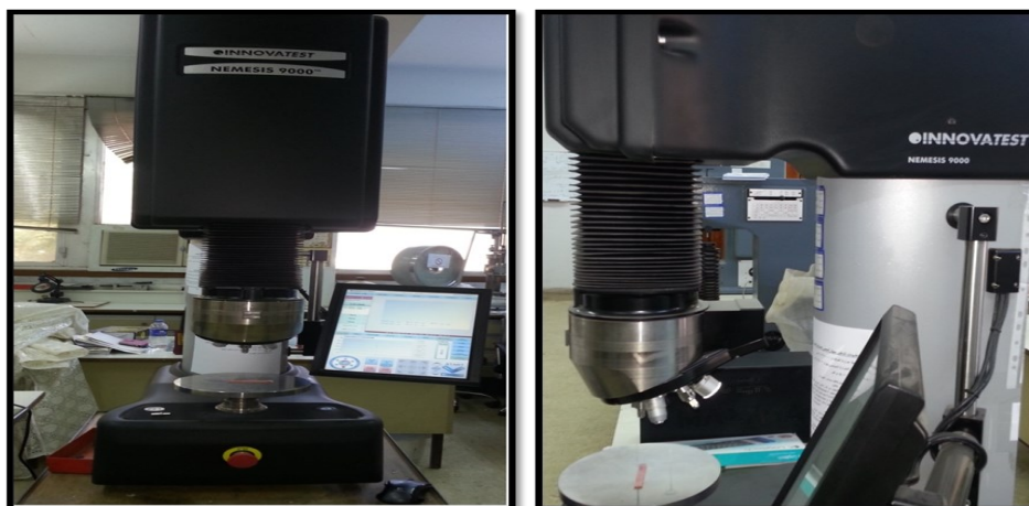
Figure 4: Digital general hardness tester (INNOVATEST. Company NEMESIS) Model no 9001, 2012
