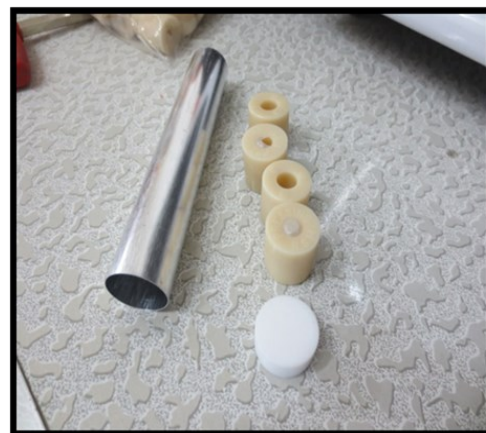
Figure 1: Large vertex cartridge, acetal discs, and replica
