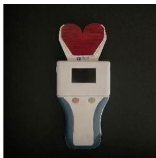
Figure 4: OccluSense (digital occlusal analysis device)
