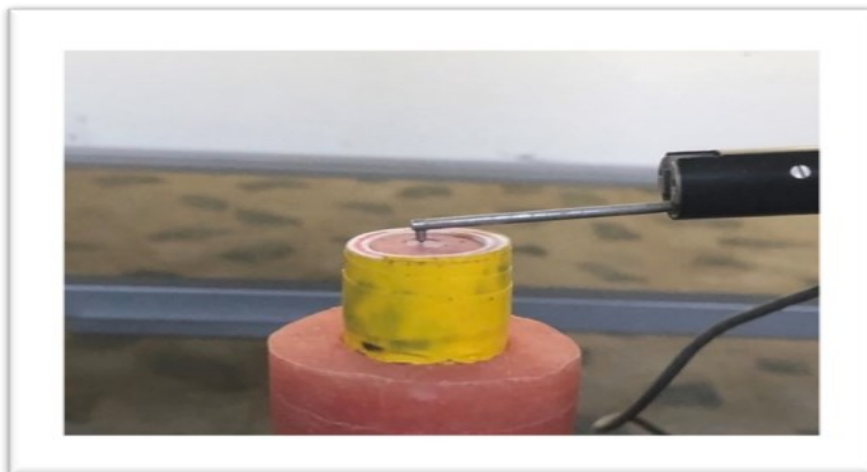
Figure 7 : Surface roughness testing by using Taylor Hobson profilometer head.
