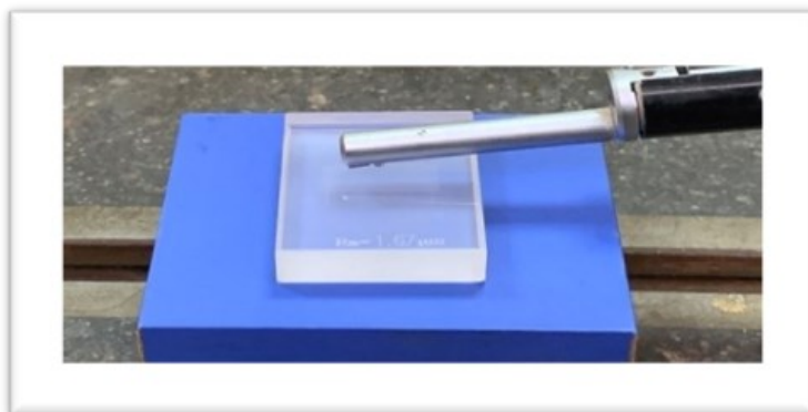
Figure 8 : Calibration of the profilometer by using 1.64\mu\text{m} block.
