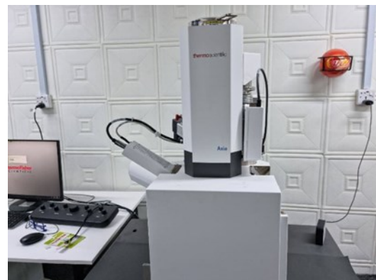
Figure 2: Scanning electron microscope used for smear layer removal evaluation test
