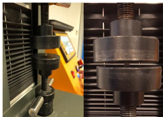
Figure 4. Universal testing machine, compressive strength test
