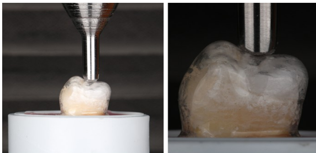
Figure 3. Custom Ethylene Vinyl Acetate Copolymer coverage of the occlusal surface during the loading procedure
