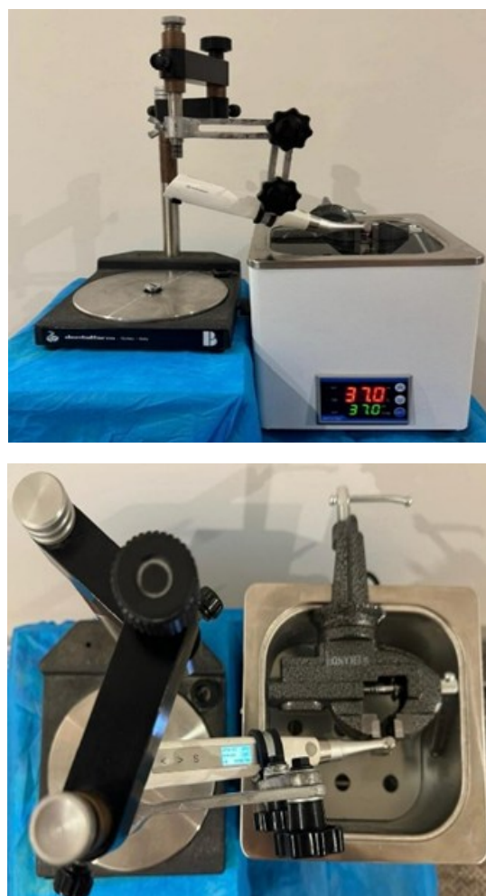
Figure 3A, Figure 3B Resin block instrumentation using dental surveyor with an endodontic engine is mounted in a water bath
