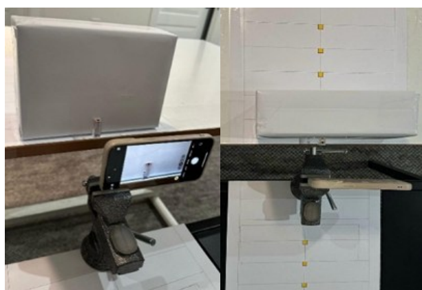
Figure 2. Photographing of resin blocks using a standard camera position
