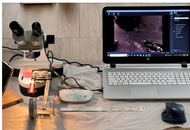
Figure 4. Marginal fit test with stereomicroscope 40x and Hayear camera software
