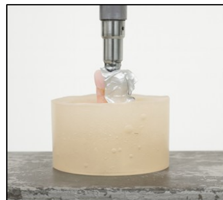
Figure 14. Tinfoil placed between loading ball and sample
