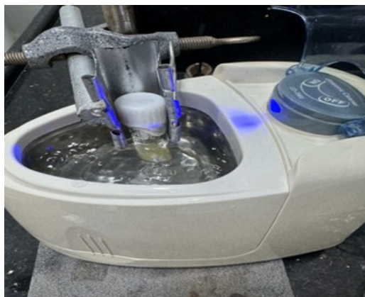
Figure 2. Mixing of Metapex with ZnO Nanoparticles by ultrasonic sonicator
