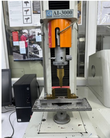
Figure 3. Three-point bending test for Flexural strength
