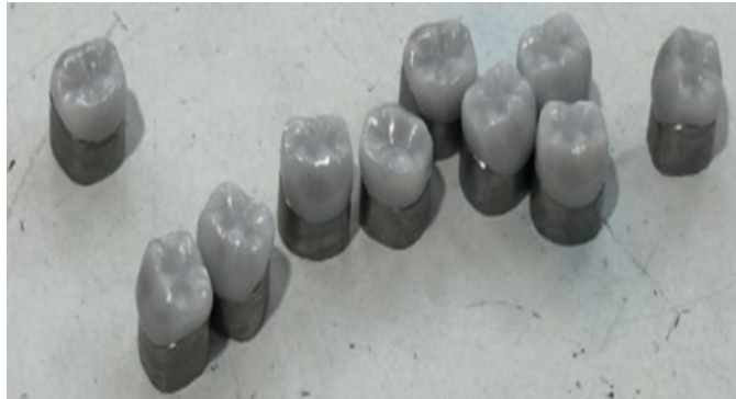
Figure 1. Ten monolithic full anatomic zirconia crowns after cementation and before testing
