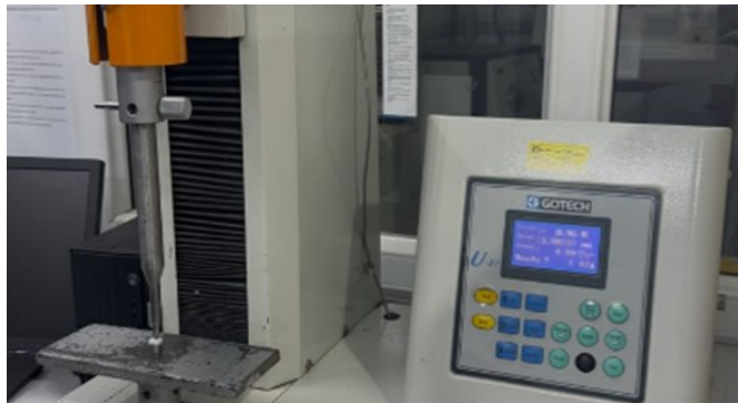
Figure 2. The universal load testing machine was used while testing the monolithic full anatomic zirconia crowns
