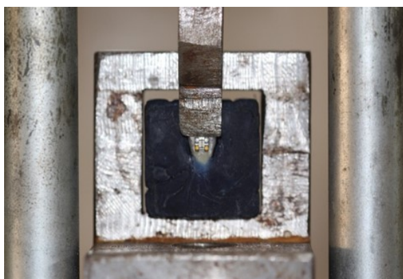
Figure 3: Application of occluso-gingival load
