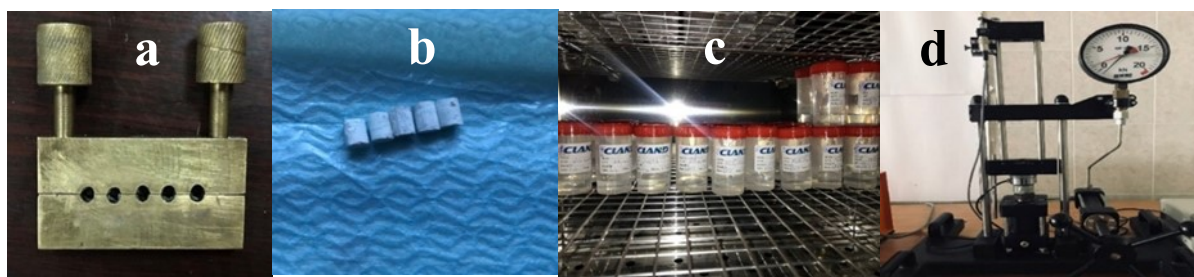
Figure 2: (a) Stainless steel mold, (b) Specimens, (c) Specimens in distill water, (d) Universal machine.
