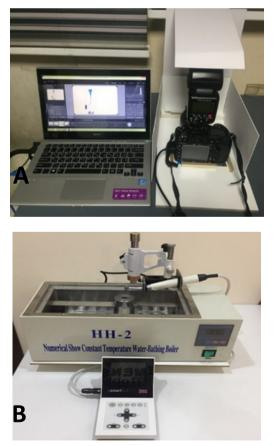
Figure 1: A- Imaging of resin blocks with the standardized position of digital camera. B- Cylinder shaped steel holder inside a water bath fixed to dental surveyor with endo motor.
