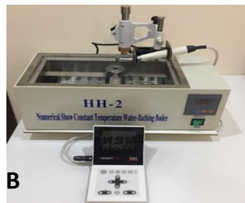
Figure 1: A- Imaging of resin blocks with the standardized position of digital camera. B- Cylinder shaped steel holder inside a water bath fixed to dental surveyor with endo motor.
