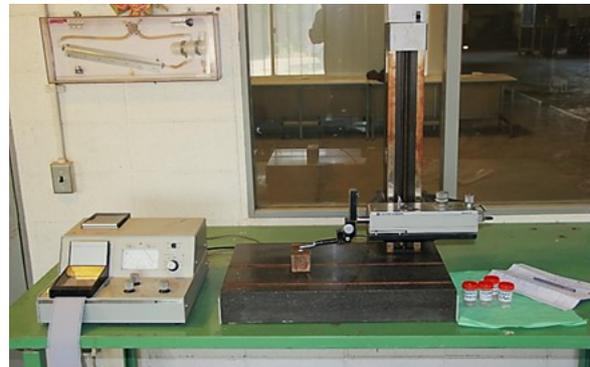
Figure 5: "Profilometer" for surface roughness testing.
