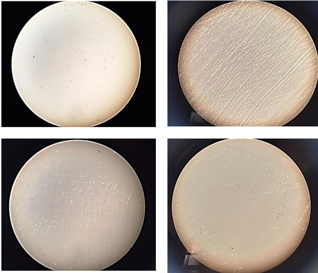
Figure 6: Stereomicroscope images of zirconia samples at x250 of GA: Control group, GB: Grinded group, GC: Reglazed group and GD: Polished group.
