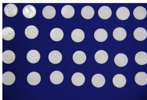
**Figure 2: Glazed zirconia discs.**
