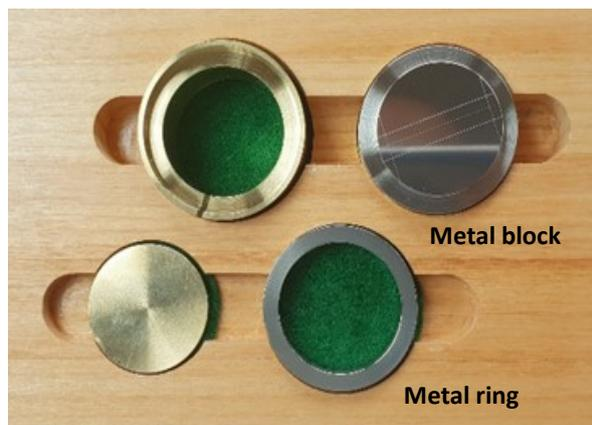
Figure 2: ADA specification number 19 apparatus used in the study.
