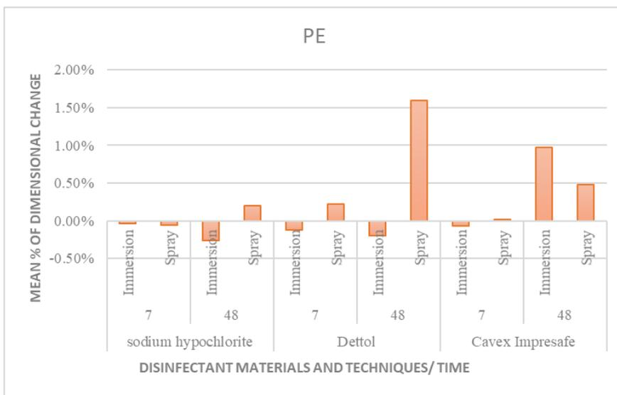
Figure 7: Mean values of dimensional changes for PE material.
