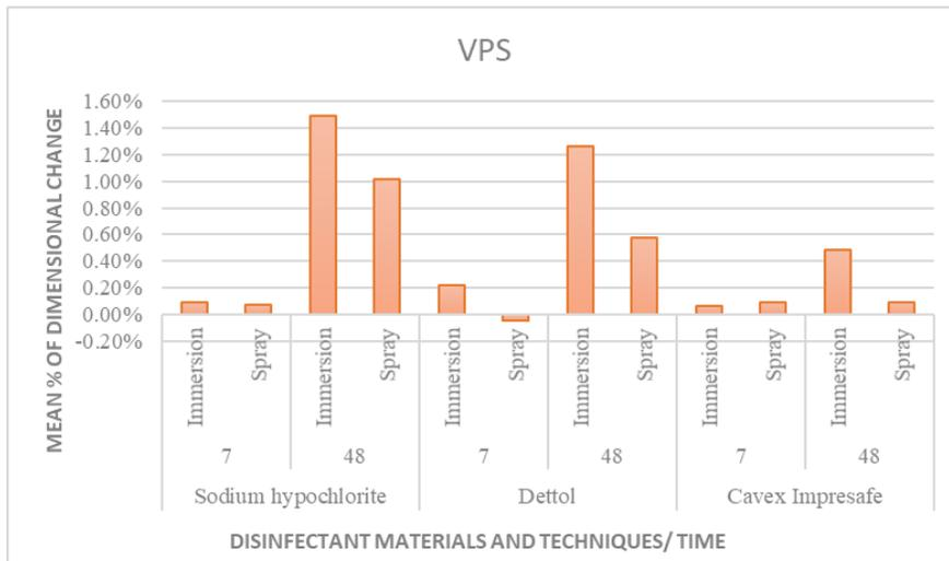
Figure 6: Mean values of dimensional changes for VPS material.
