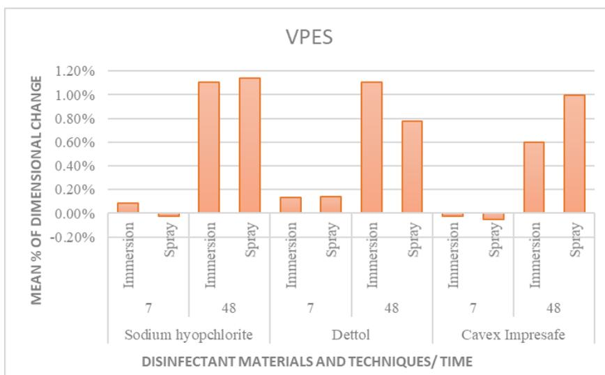
Figure 8: Mean values of dimensional changes for VPES material.
